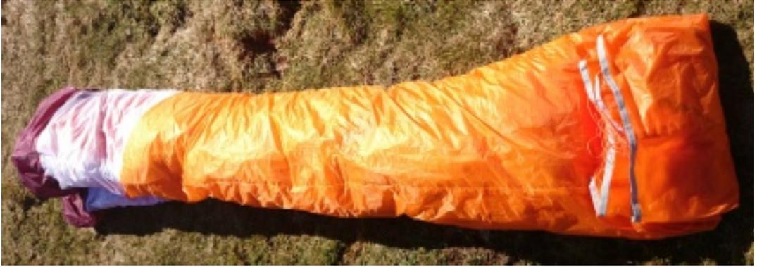
Fold your wing aligning the leading edge of rushes and leave only one cell width. Make a first ply 25 cm above the trailing edge so as not to bend the rods located in upper .
